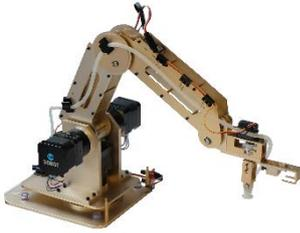
picture 10: OMiarm1 - Dobot arm v1.0 with vacuum suction cap and pen holder
