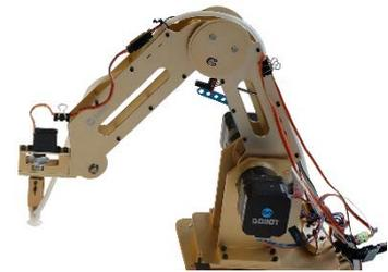
picture 11: OMiArm2 - Dobot arm v1.0 with vacuum suction cap
